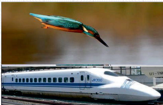
Figure 1.5 Bullet train noses imitate the beak of a kingfisher
